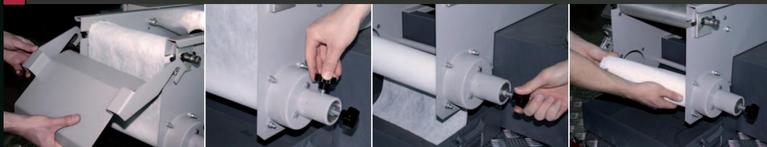
QUICK AND EASY SUBSTITUTION OF THE FILTERING MATERIAL.
