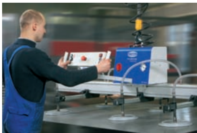
VacuMaster Comfort, 750 kg maximum load, horizontal
