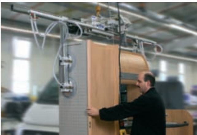
VacuMaster Box, 200 kg maximum load, for installation of kitchen elements in mobile homes
