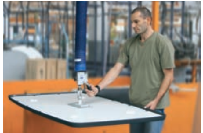
JumboHandy, maximum load 30 kg, with single suction pad for commissioning camping tables
