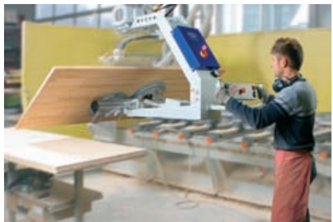
VacuMaster Comfort, maximum load 125 kg, with 180° turning, for loading CNC machines with sheets of glued wood
