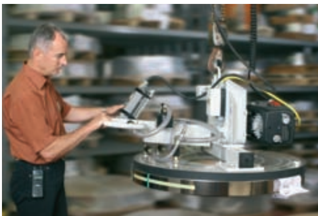
VacuMaster Coil, maximum load 750 kg, horizontal, for handling stainless-steel coils
