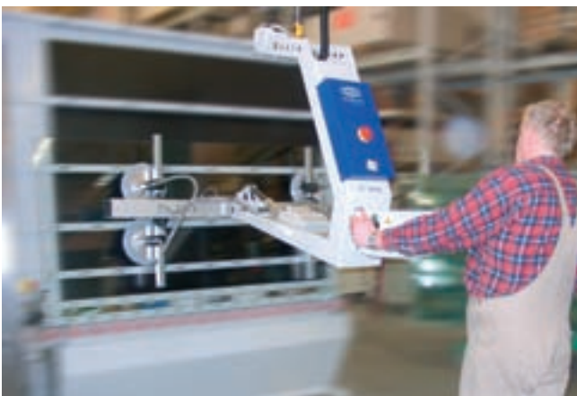
VacuMaster Comfort, maximum load 125 kg, with 180° turning, for handling panes of glass
