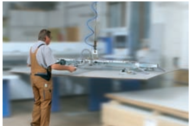
VacuMaster RE, maximum load 250 kg, for loading machine tools
