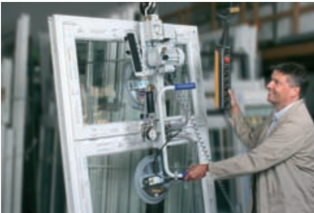
VacuMaster Window, maximum load 170 kg, vertical, for handling of multi-casement windows
