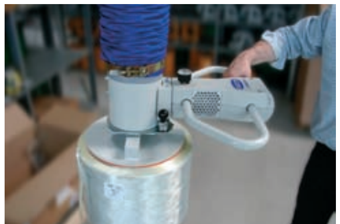
JumboErgo, maximum load 65 kg, with round suction pad, for handling rolls of plastic film
