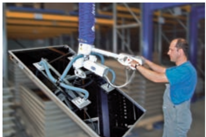
JumboErgo, maximum load 70 kg, with pneumatic swivelling unit, for lifting solar modules in a horizontal position and placing them vertically on a commissioning trolley
