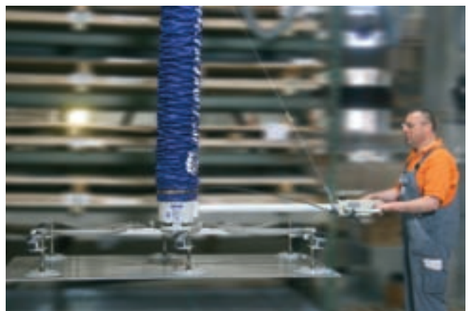
JumboErgo, maximum load 140 kg, for commissioning small and medium-sized sheets of aluminum
