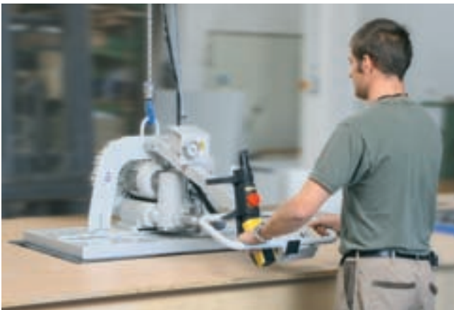
VacuMaster Multi, maximum load 400 kg, horizontal, for loading a sheet saw with large sheets of wood
