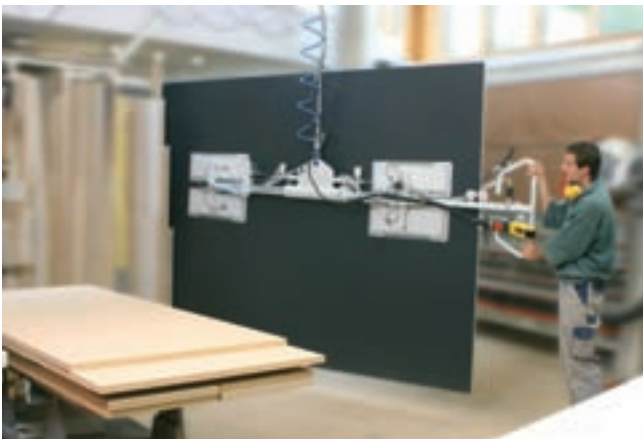
VacuMaster HHVM, maximum load 200 kg, swivelling by +/- 90°, for removing sheets from vertical storage racks
