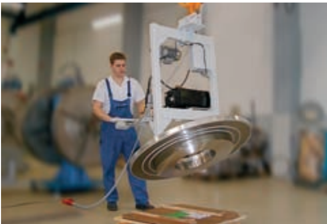
VacuMaster Coil, 750 kg maximum load, with 90° swivelling, for handling coils and rings of split strip
