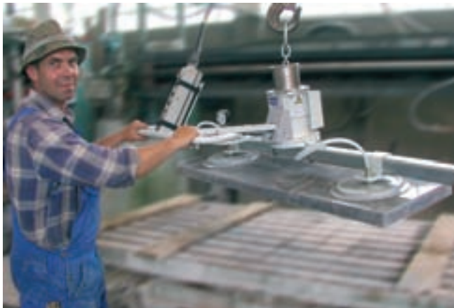
VacuMaster Eco, maximum load 250 kg, horizontal, for loading and unloading of stoneworking machines
