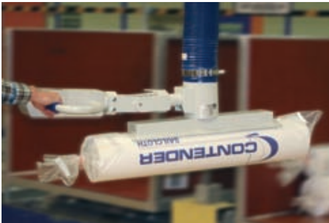
JumboErgo, maximum load 45 kg, for commissioning rolls of textile materials packed in plastic film
