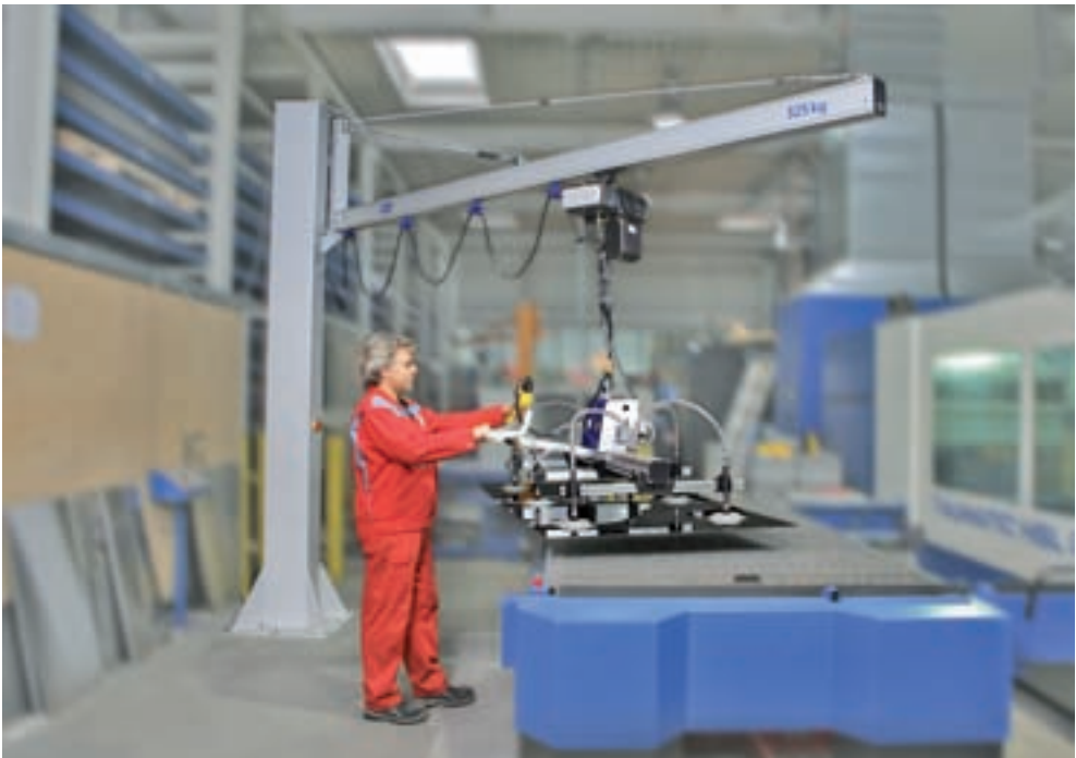
VacuMaster Basic, maximum load 250 kg, horizontal, for handling sheets of stainless steel
