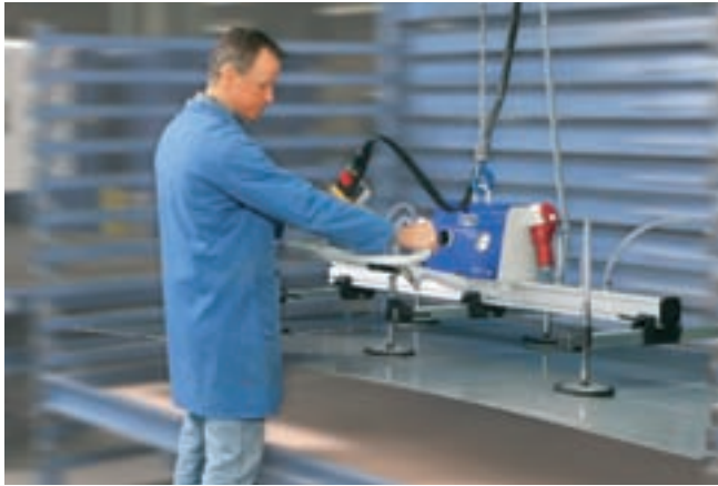
VacuMaster Basic, maximum load 250 kg, horizontal, for loading and unloading steel racks
