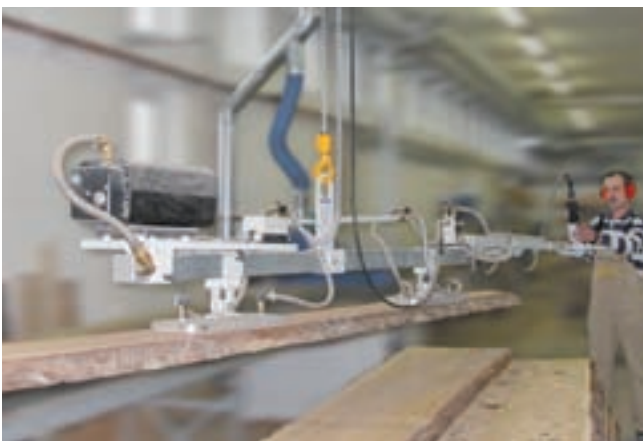
VacuMaster VHB, maximum load 500 kg, for handling of rough-sawn planks
